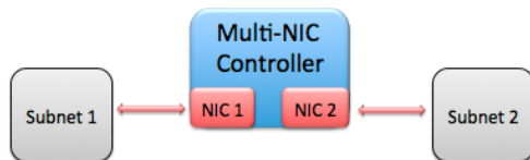
Figure 4. When configuring a controller with multiple NICs, each NIC should communicate with a different subnet. Configuring two or more NICs on the same subnet may cause communication problems.
